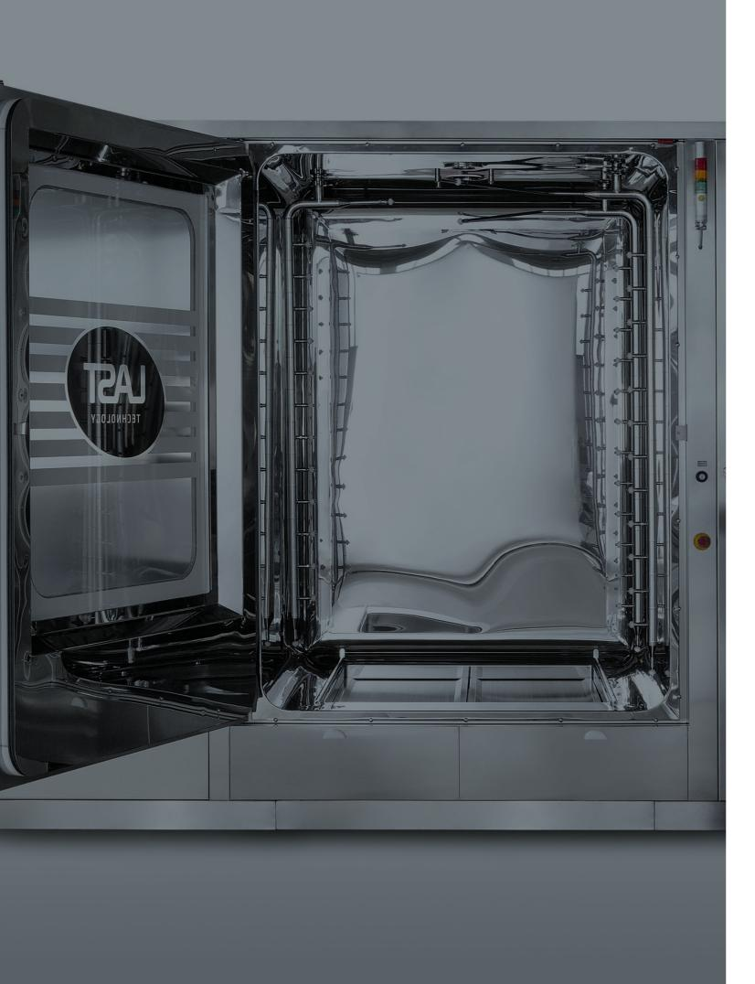
LAST Technology's engineering team was entrusted to design a high-efficiency machine that could increase washing efficiency by dissolving encrustations and active pharmaceutical ingredient (API) residue from flat surfaces, such as trays and frames. More specifically, this pharmaceutical company manufacturers steroid solutions.
